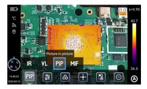
**PIP** – picture in picture – both infrared and visual images are displayed.
