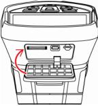
Close the slot cover and slide it in the arrow direction shown until it is locked.
