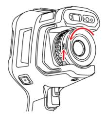
Press the lens changing button and rotate the lens anticlockwise and take it off.
